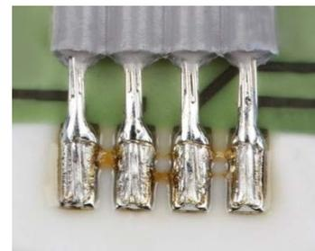
Figure 15 The hot bar imprint on the surface of the wires is a good indicator of how well a joint has been formed
