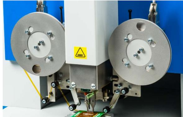
Figure 4: Kapton tape on interposer module
