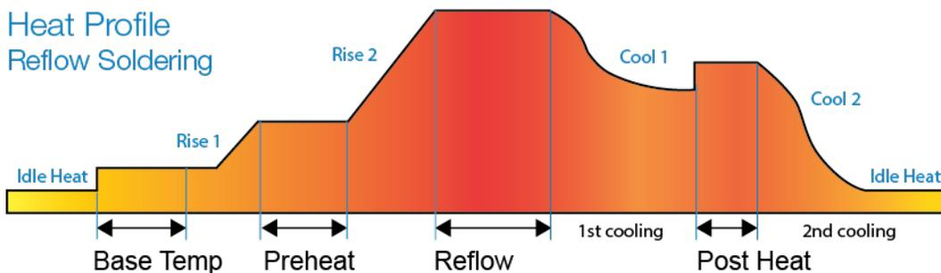
Figure 9 Heat Profile - Reflow Soldering
